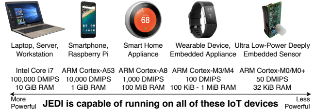
Figure 1: IoT comprises a diverse set of devices, which span more than four orders of magnitude of computing power (estimated in Dhrystone MIPS). 1
